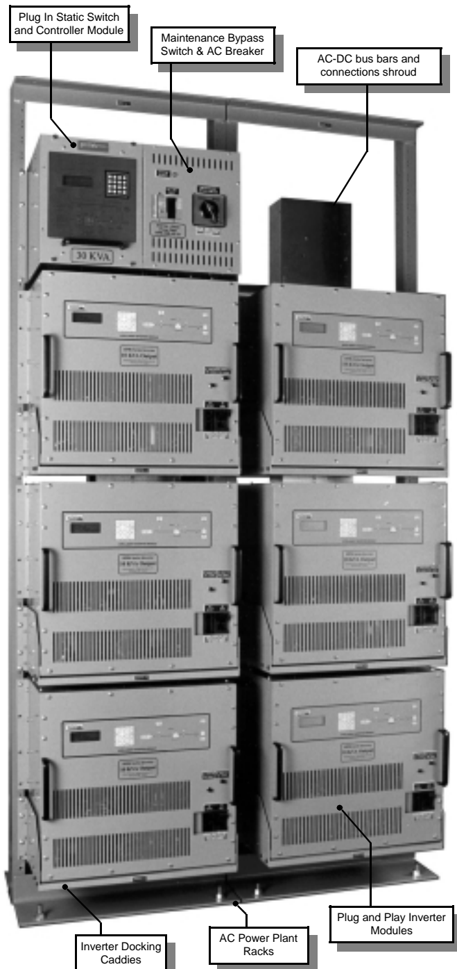
Inverter System as shown above: 30 kVA 3 Phase Dual Redundant Output
